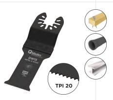
Wide range of applications due to Bi-metal teeth. Length to holder 54mm. Thickness 0.8mm.
