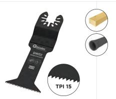
Coarse set teeth for easy plunge cuts in material at any location. Length to holder 68mm. Thickness 0.6mm.
