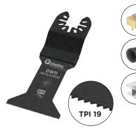
Wide range of applications due to Bi-metal teeth. Length to holder 57mm. Thickness 0.8mm.
