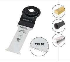
Wide range of applications due to Bi-metal teeth. Length to holder 42mm. Thickness 0.8mm.
