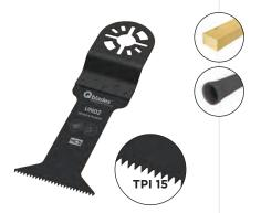
Coarse set teeth for easy plunge cuts in material at any location. Length to holder 68mm. Thickness 0.8mm.
